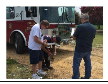
An open window reading that is <u>higher</u> at 3 ft. (probe face up) than at 3 in. (probe face down) Plume is Overhead
