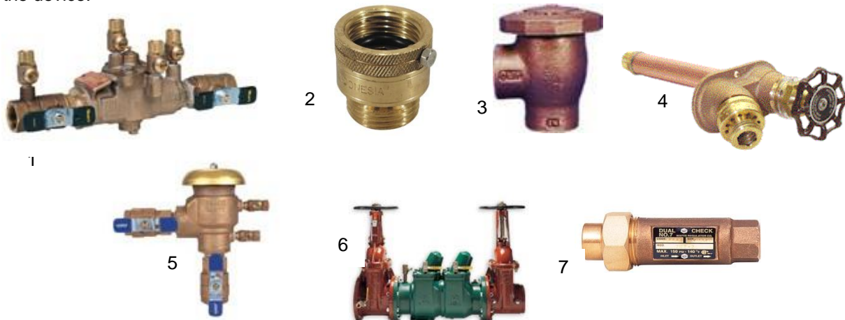
(1) Reduced pressure principle backflow prevention assembly (RPZ) (2) Hose bibb vacuum breaker (3) Pipe applied atmospheric vacuum breaker (4) Wall hydrant with hose bibb vacuum breaker (5) Pressure vacuum breaker assembly (6) Double gate – double check assembly (7) Dual check valve
